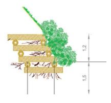
Once the different levels of the cribwall are constructed, they are filled with well-compacted soil (without mechanical systems but avoiding air spaces). At the same time, we plant and also consolidate the fronts seen between trunks with a fascine but resistant enough to hold the ground.
