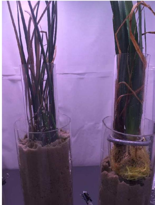
On the left, macrophyte has been transplanted into the sterile column. On the right, it can be observed that the macrophyte roots are placed beneath and surrounded by the irrigation tubing (silver tube), prior to being covered by sand.
