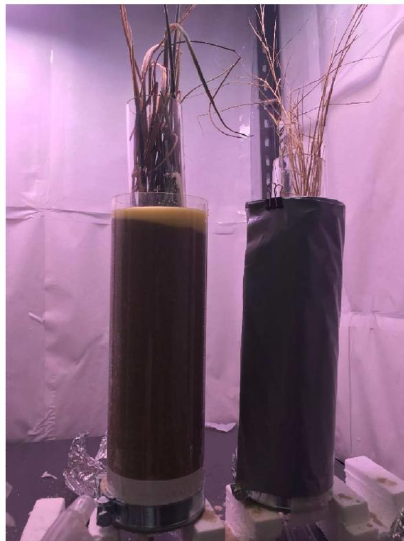
On the left, lanolin-paraffin mixture is used to seal the macrophyte. On the right, the column is covered in an opaque plastic material to hinder algal growth.
