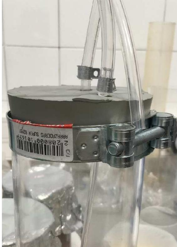
Assembly of the irrigation and extraction tubings.
