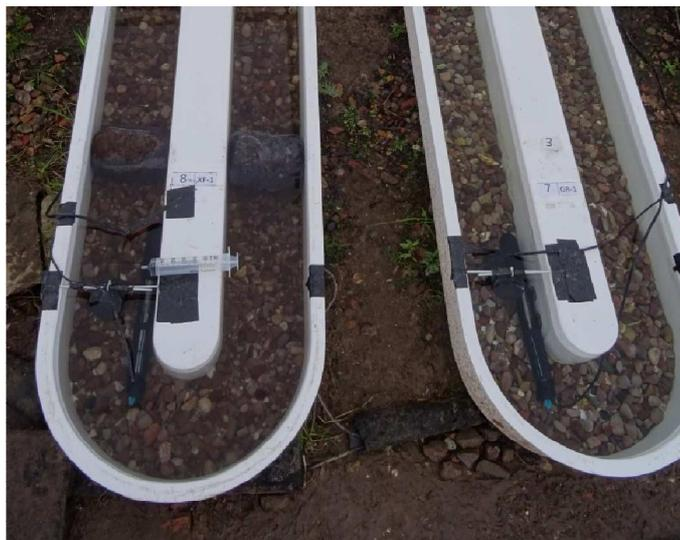
Figure 1: On the right, detail of one of the flumes with xylit mesh packs; on the left a control flume that just contents the gravel bed.
