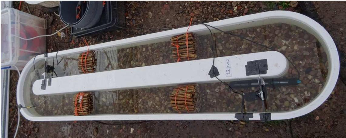
Figure 2: Flume with the four hazel twig bundles.
