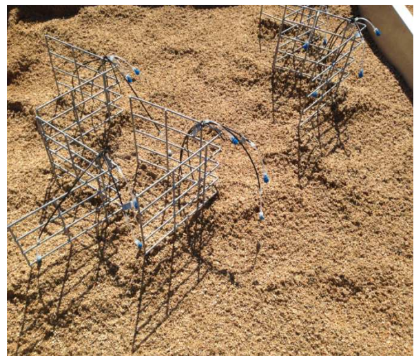
Rhizon samplers installed in the tanks
